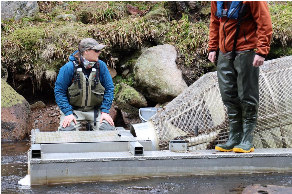
The River Dee team checks one of the River Muick rotary screw traps
